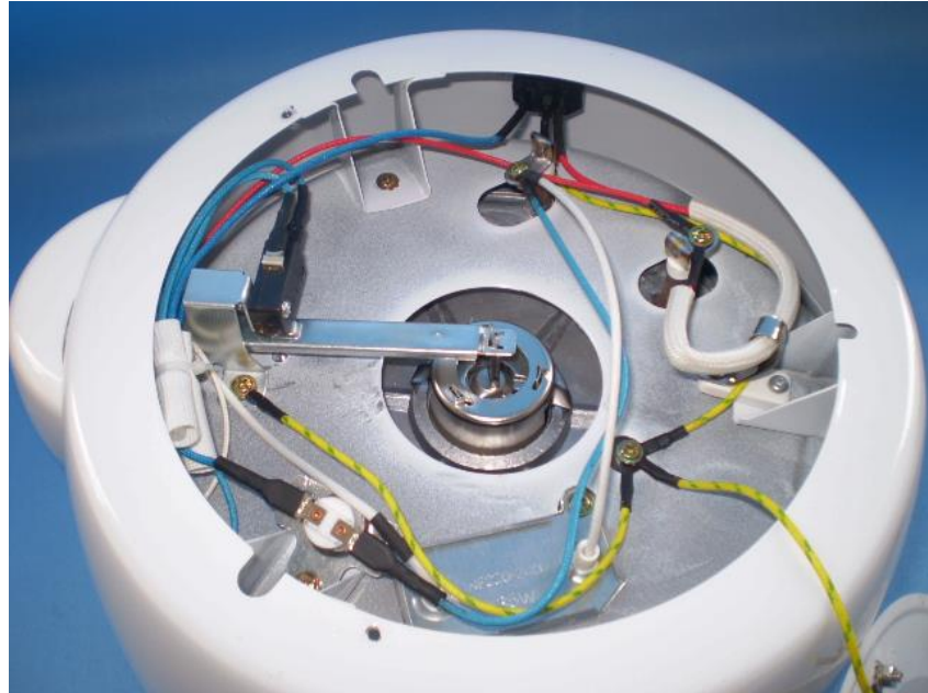
Fig. 11: Inner view, appliance inlet used and temperature limiter Y with micro switch
