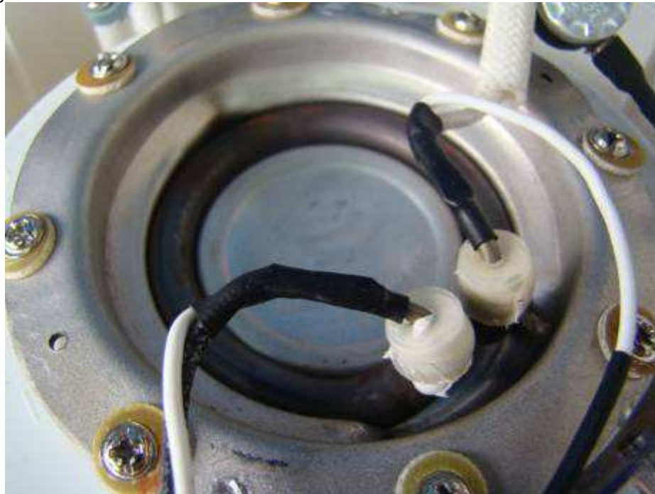
Note: The Heating element is clamped by the metallic plate
