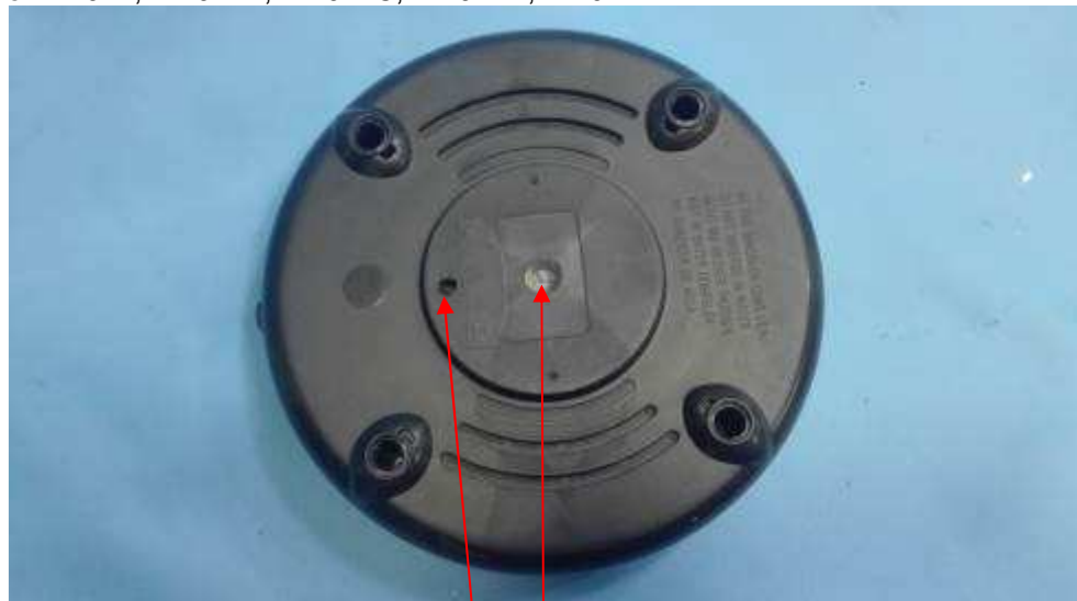
Note: Marking label on bottom enclosure Drain holes 5,2 mm in diameter
