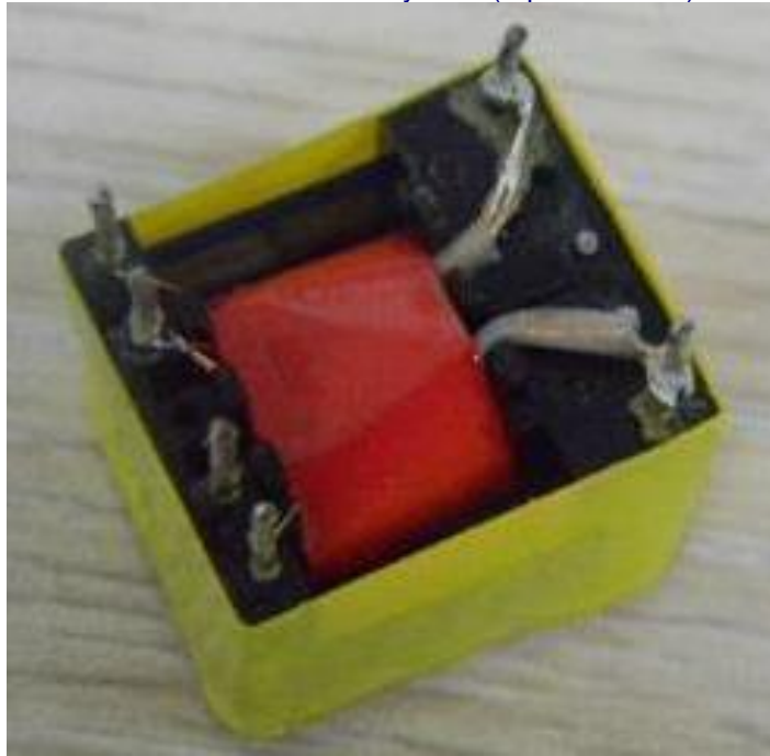
Transformer disassembly view (representative)
