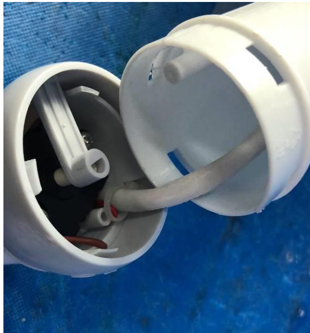
Internal view of speed switch
