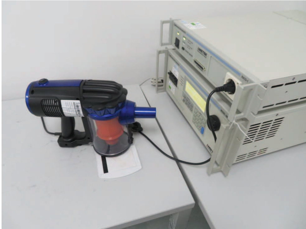
Photograph 2: Set-up for Disturbance Voltage on AC mains terminal
