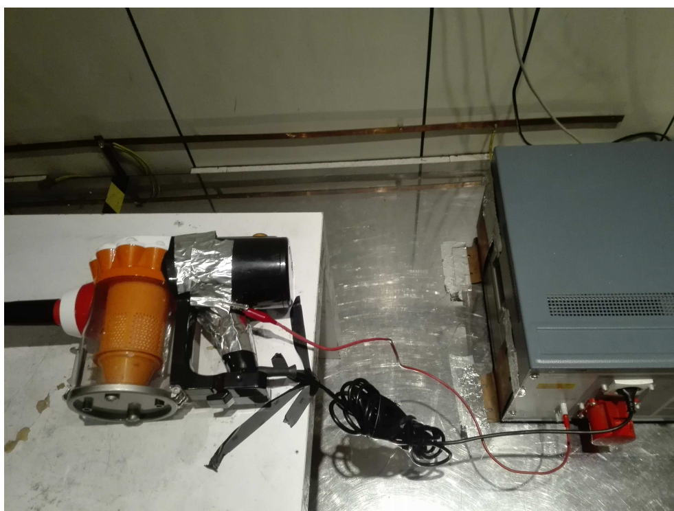
Photograph 2: Set-up for Continuous Disturbance Voltage
