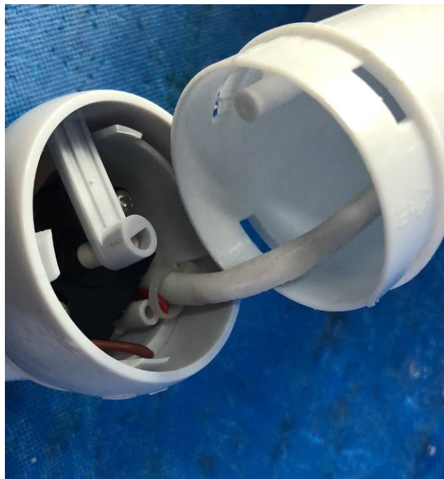
Internal view of speed switch
