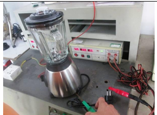
60. Earthy continuity test
