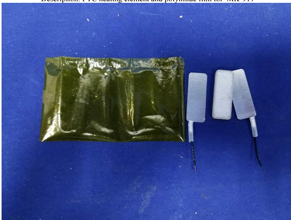
Photo 20 Description: PTC heating element and polyimide film for MK-919
