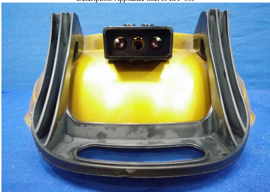
Description: Appliance inlet of EFP-005
