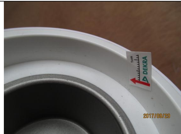
62. Defect: Dirty mark on housing - Minor
