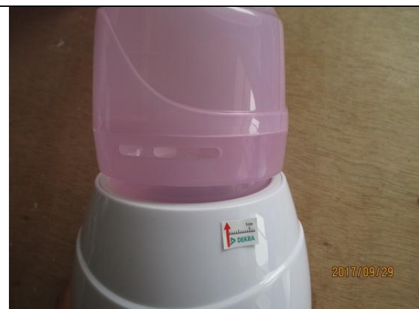
60. Defect: the nasal mask not fixed on body firmly - Major
