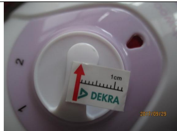
64. Defect: Dirty mark on housing - Minor
