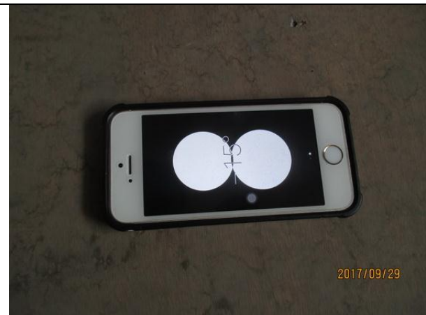
58. Stability test at 15°
