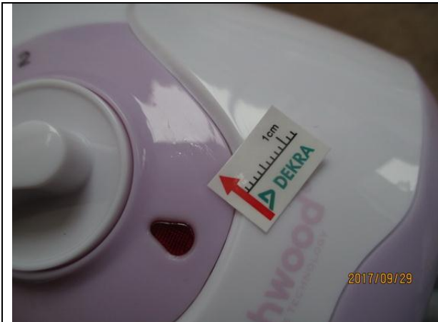
61. Defect: Scratch mark on housing - Minor
