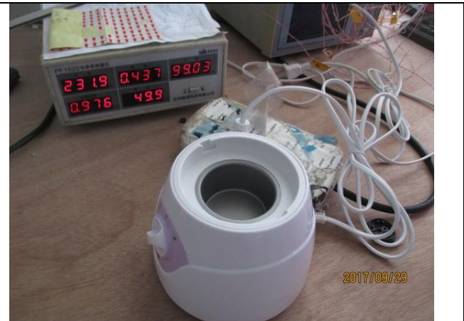
50. Power input test
