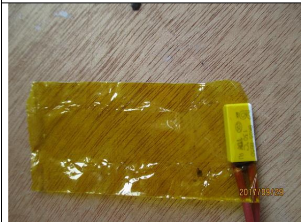
45. Thermal cut-out (3-layer)
