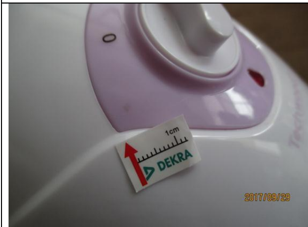
63. Defect: Dirty mark on housing - Minor
