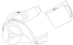
3. Garbage disposal: Press buckle and open the bottom of the dust cup.
