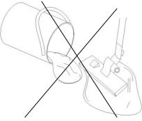
5. Do not suck in needles, drawing-pins or string cement, plaster, or other material for construction and decoration.
