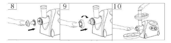
Place the accessories for the meatballs on the shaft of the feed screw, adjust by turning to insert the pins into the slots (fig.8).
