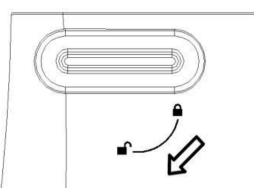
Install the bowl lid (1) on the spindle. Turn clockwise to secure.
