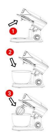
Install the accessory (whip or hook or beater) on the axis of the robot by engaging it in the axis (3). Turn counter-clockwise (left) to lock.
