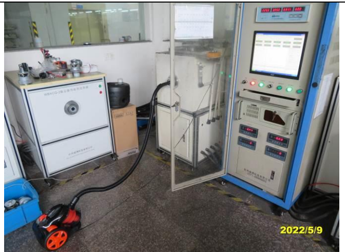
116. Full function test (suction power, airflow)
