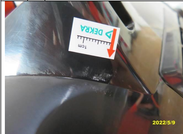
125. Dirty mark on surface-minor TAS-759
