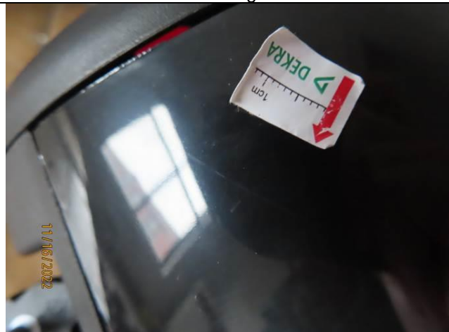
82.Minor - Scratch on housing.
