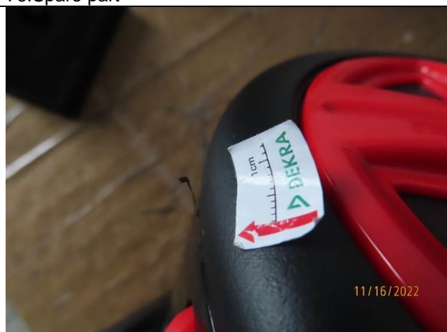
78. Minor - Soft burr on housing.
