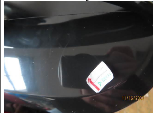
81.Minor - Scratch on housing.
