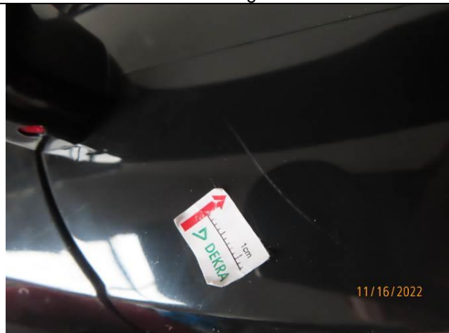
84.Minor - Scratch on housing.
