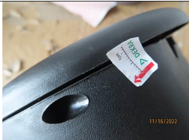
80.Minor - Scratch on housing.
