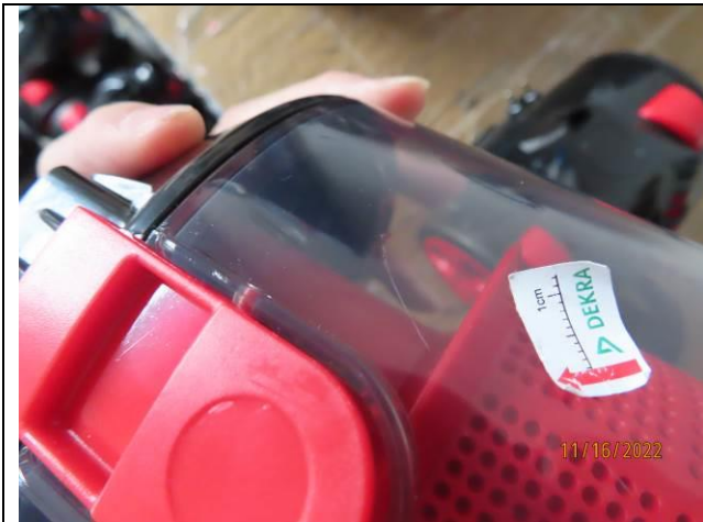
79.Minor - Scratch on housing.
