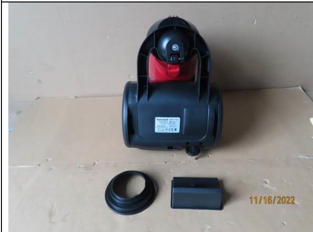
27.Plastic protection part detached
