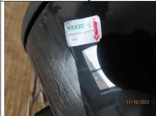
83.Minor - Scratch on housing.
