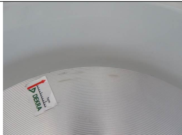
245. Stain mark on heating plate
