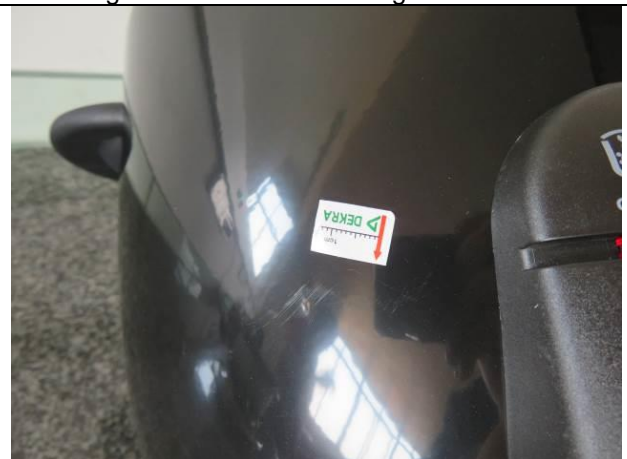
250. Slight scratch mark on housing
