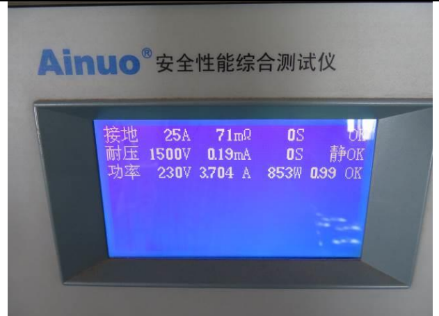
230. Hi-pot / earth resistance test and power consumption measurement
