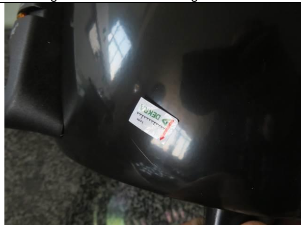
251. Slight scratch mark on housing
