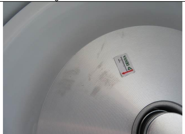
246. Stain mark on heating plate
