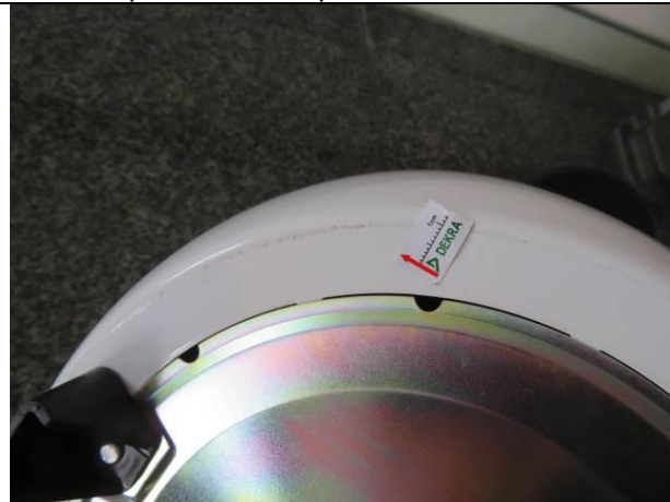
247. Stain mark on housing
