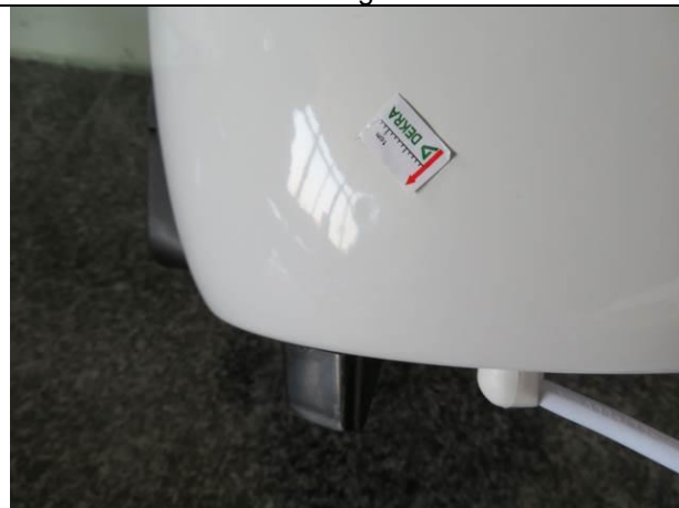
249. Slight dent mark on housing
