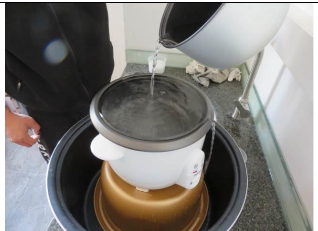
244. Over filling check
