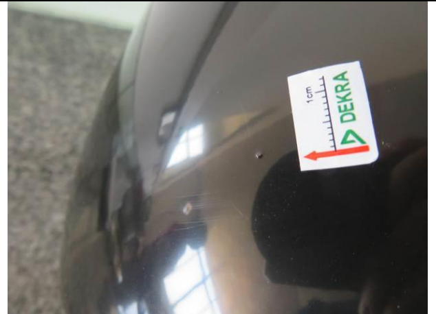
254. Poor painting on housing
