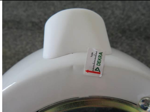
253. Slight dent mark on housing
