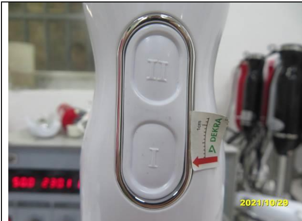
205. TMS-9600, Soft pad on switch is askew – major
