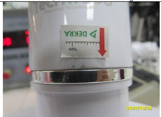
210. TMS-9600, Dirt mark on housing –minor
