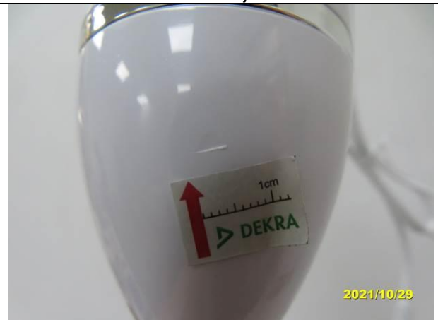
208. TMS-9600, Scratch mark on housing –minor
