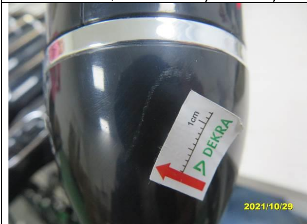
203. TMP-666, Scratch mark on housing –minor
