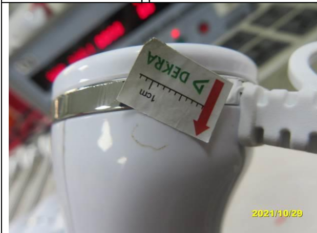
201. TMP-660, Dirt inside of injection –major
