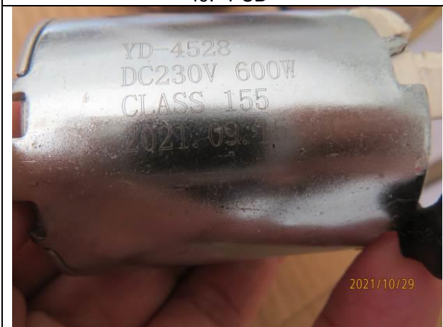
51. Marking on motor
