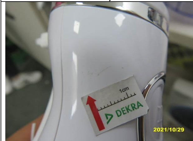
207. TMS-9600, Scratch mark on housing –minor
