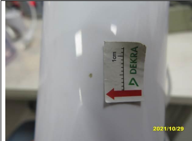
211. TMS-9600, Dirt inside of injection –major
