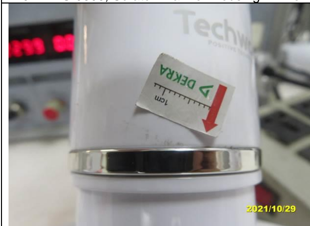
209. TMS-9600, Dirt mark on housing –minor
