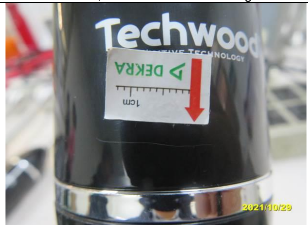
204. TMP-666, Scratch mark on housing –minor
