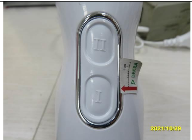
206. TMS-9600, Soft pad on switch is askew – major
