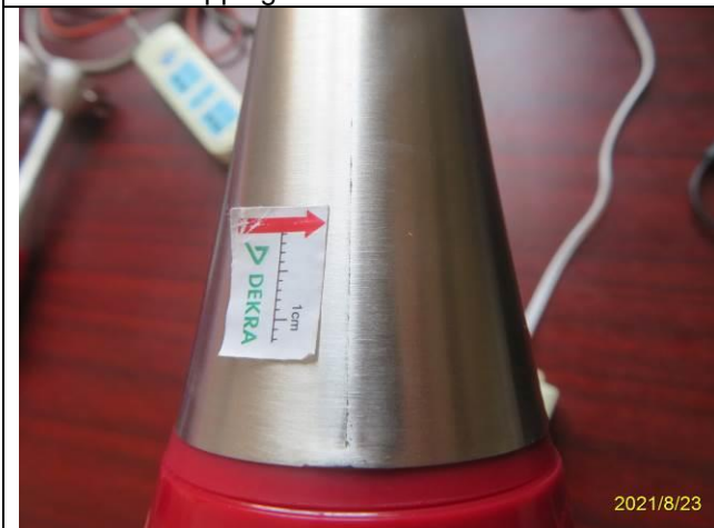
195. Defect-major-Obvious scratch mark on product(item TMS-8366)
