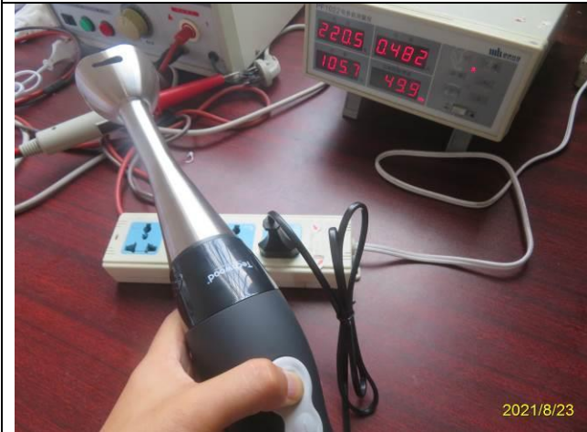
183. Power consumption check
