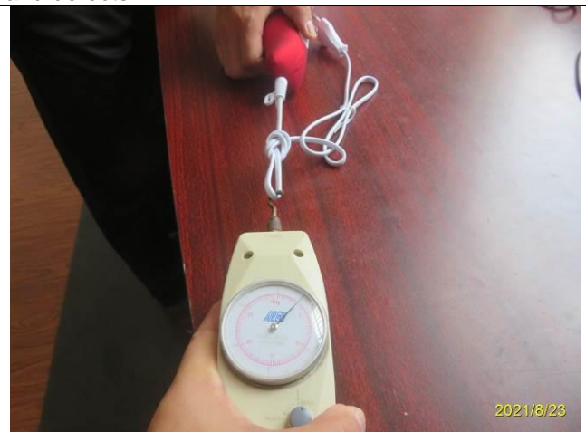
180. Strain relief test
