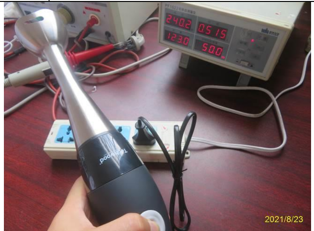
184. Power consumption check
