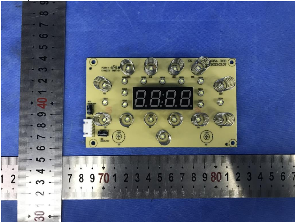
Description: Control PCB Internal view of AF-005A-1
