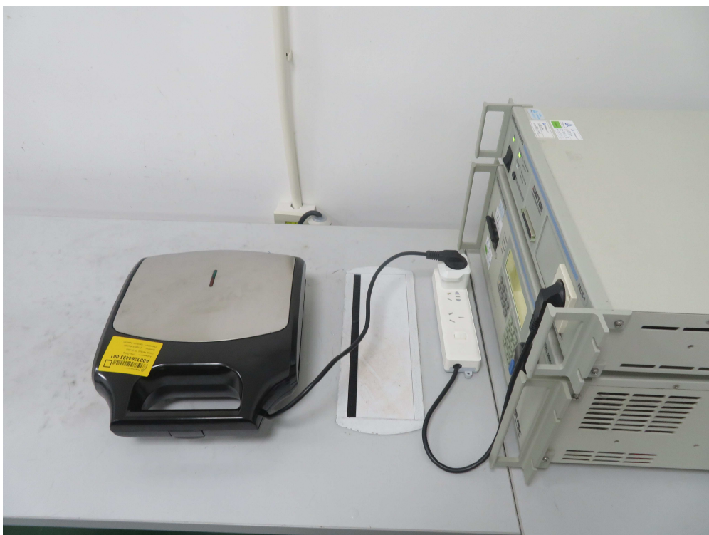
Photograph 2: Set-up for Emission of Voltage Fluctuation and Flicker
