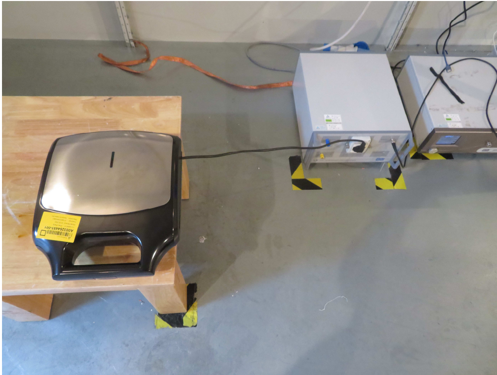
Photograph 2: Set-up for Emission of Voltage Fluctuation and Flicker
