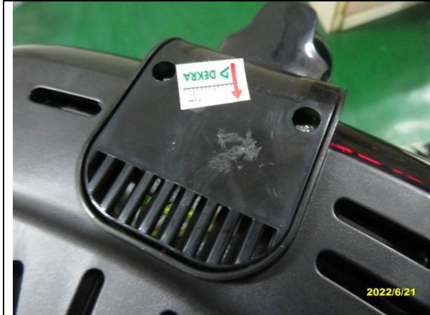
157. Dirty stain on housing –minor-TFR-456SH
