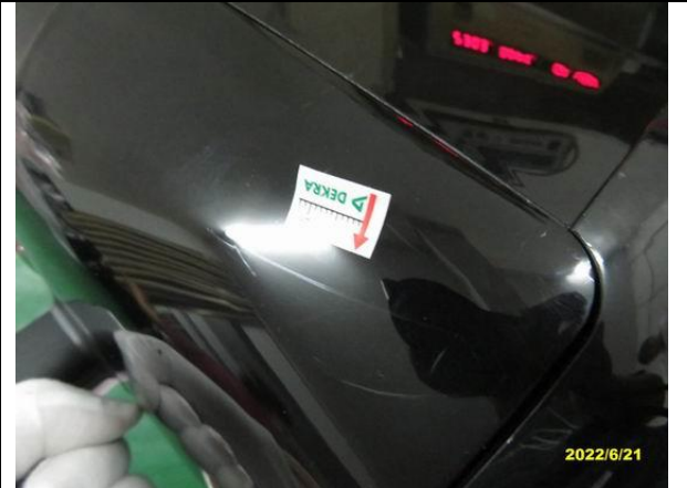
162. Scratch on housing -minor-TFR-452SHD
