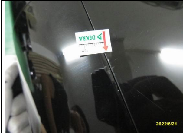
161. Scratch on housing -minor-TFR-452SHD
