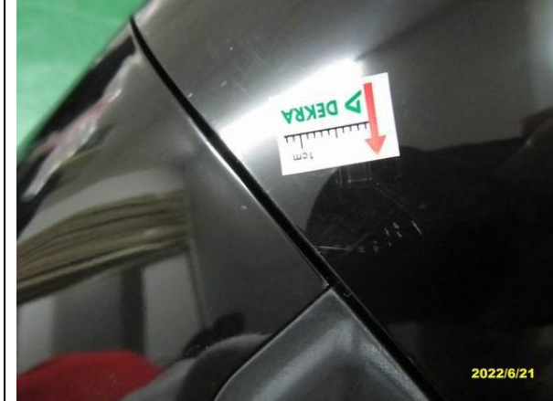
159. Scratch on housing –minor-TFR-456SH
