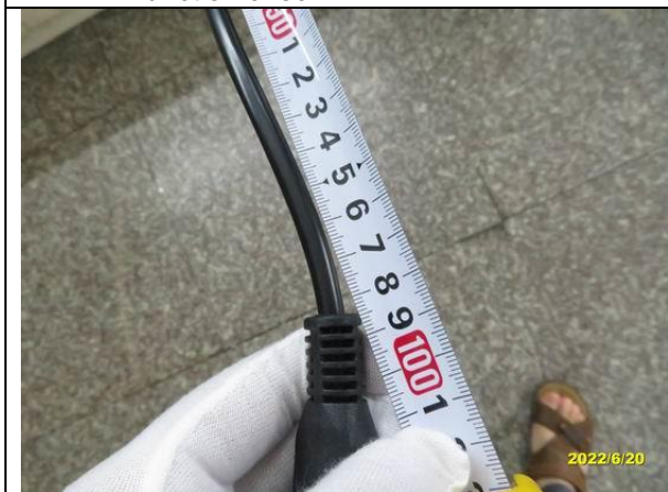
143. Power cord length check
