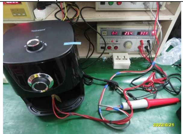
132. Earthed resistant measurement check
