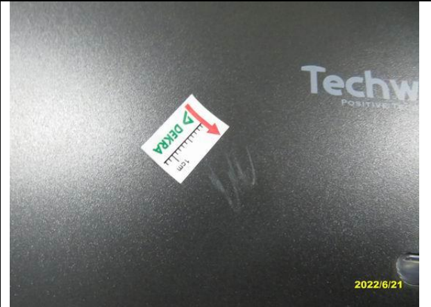
158. Scratch on housing –minor-TFR-456SH
