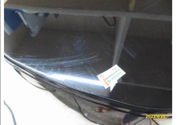
160. Scratch on housing -minor-TFR-452SHD
