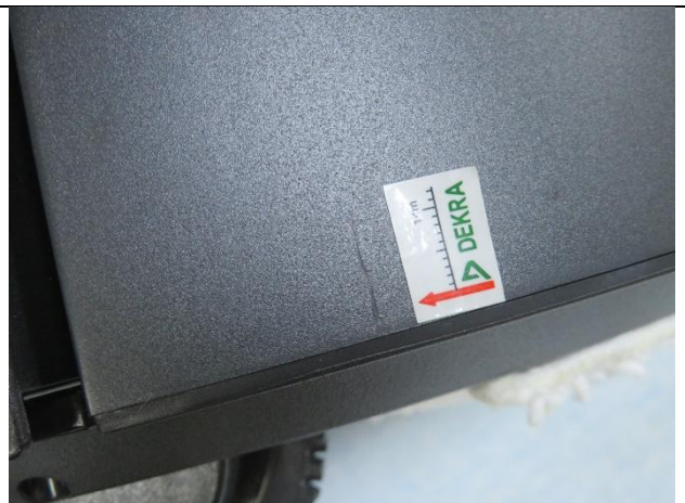
174. Scratched mark on the housing
