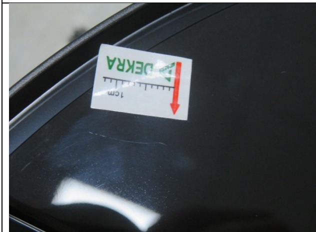
173. Scratched mark on the housing
