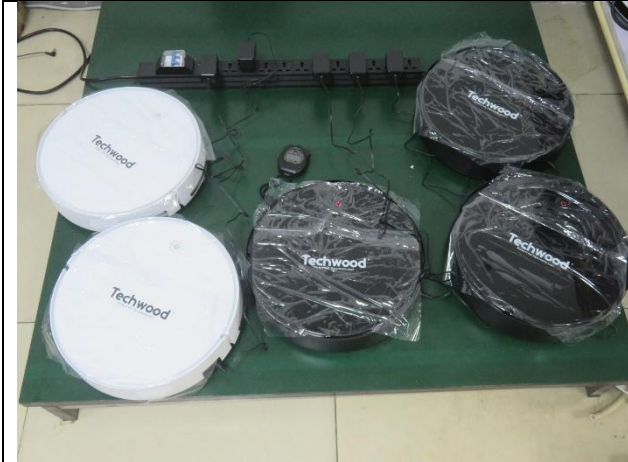
163. Endurance test (charging)
