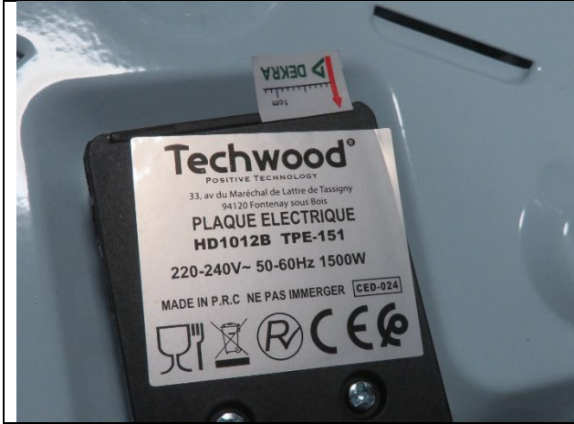
121. Poor stuck of rating label
