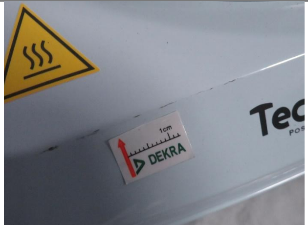
124. Dirty stain on the housing
