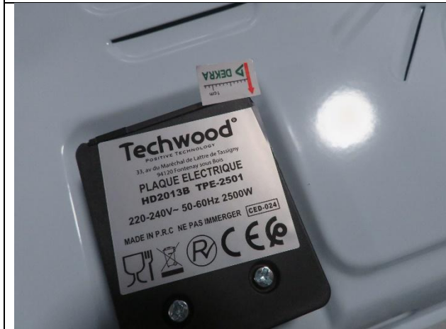
129. Poor stuck of rating label
