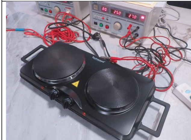
113. Earth resistance measurement
