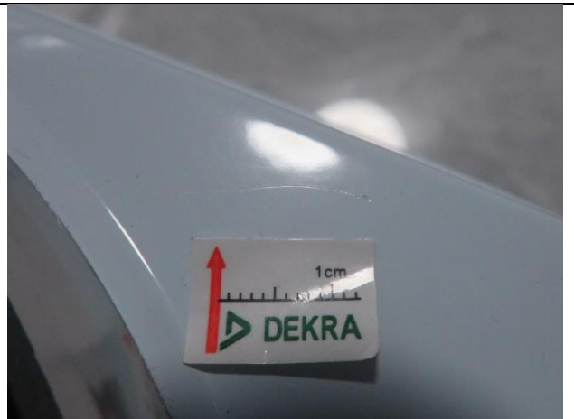
130. Scratched mark on the housing
