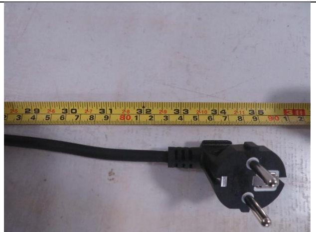
118. Power cord length measurement
