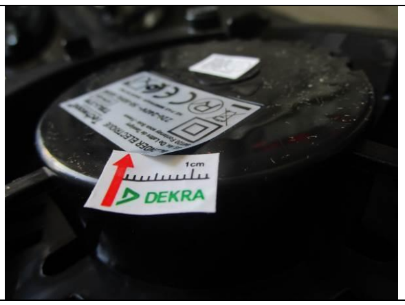
106). Poor stuck for rating label
