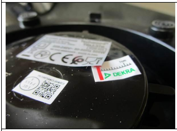
105). Poor stuck for rating label
