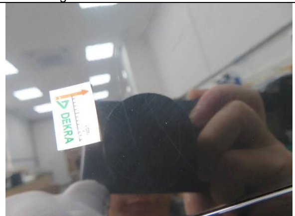
252. Minor defect: Scratch mark on the housing
