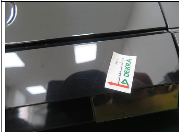
251. Minor defect: Scratch mark on the housing
