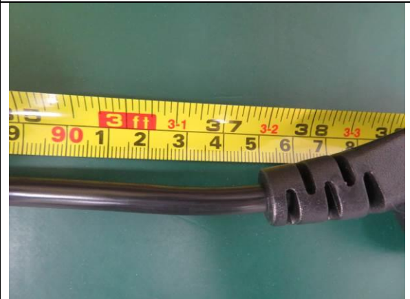
238. Power cord length check
