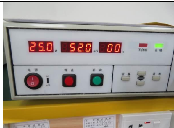
208. Earth continuity test
