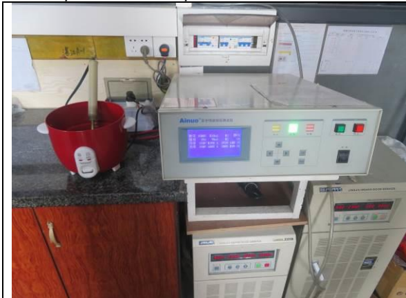
295. Hi-pot, earth continuity, keep warm power and input power consumption check
