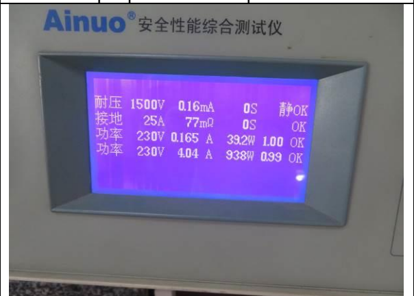
300. Hi-pot, earth continuity, keep warm power and input power consumption check
