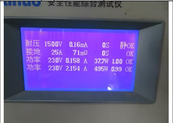
298. Hi-pot, earth continuity, keep warm power and input power consumption check
