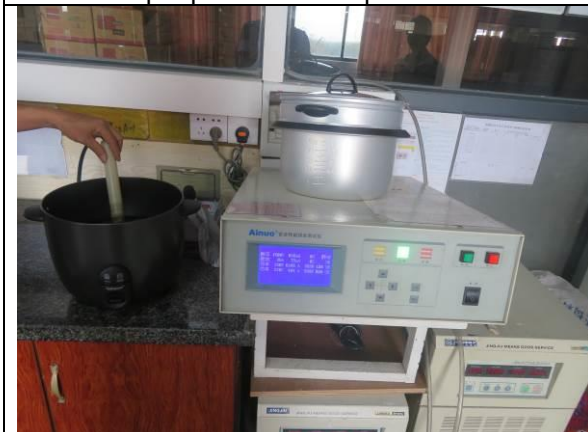
299. Hi-pot, earth continuity, keep warm power and input power consumption check
