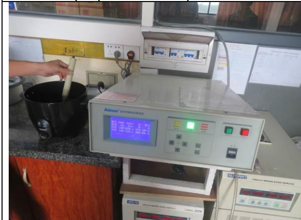
297. Hi-pot, earth continuity, keep warm power and input power consumption check
