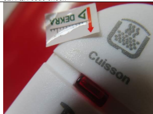
329. Minor defect: Glue residual on control panel (TCR-105)
