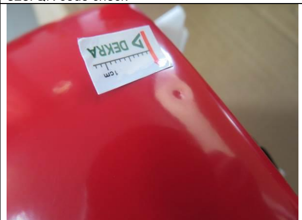
330. Minor defect: Dent mark on main housing (TCR-105)
