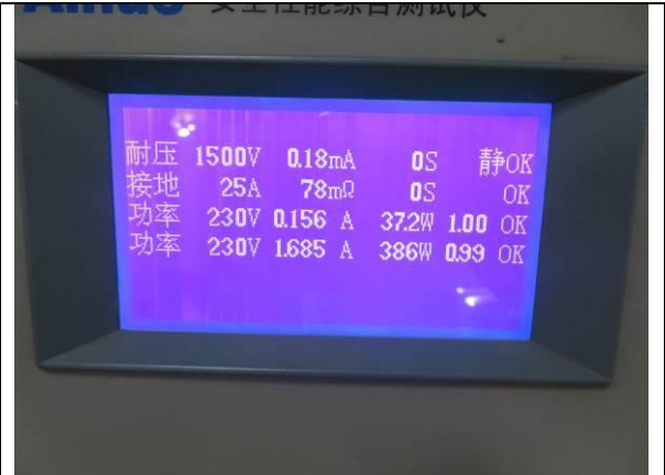
296. Hi-pot, earth continuity, keep warm power and input power consumption check
