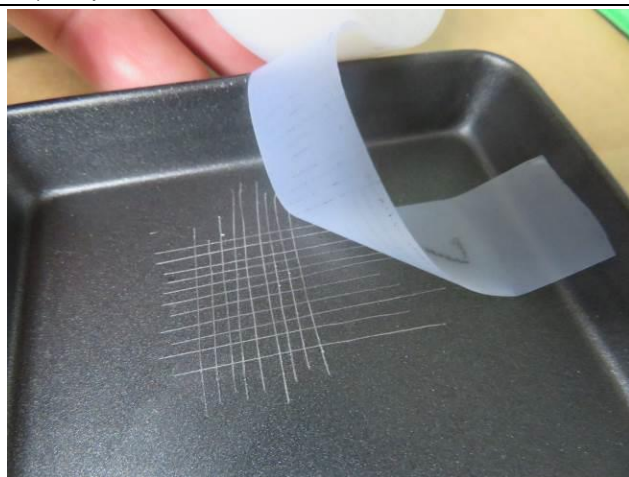
88) Coating adhesion check
