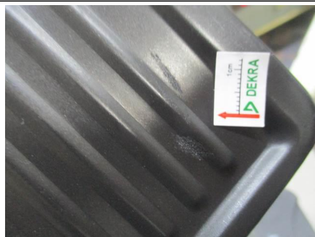
84). Poor painting of the grill
