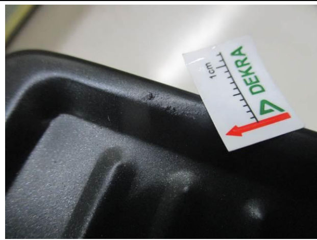
80). Poor painting of the grill
