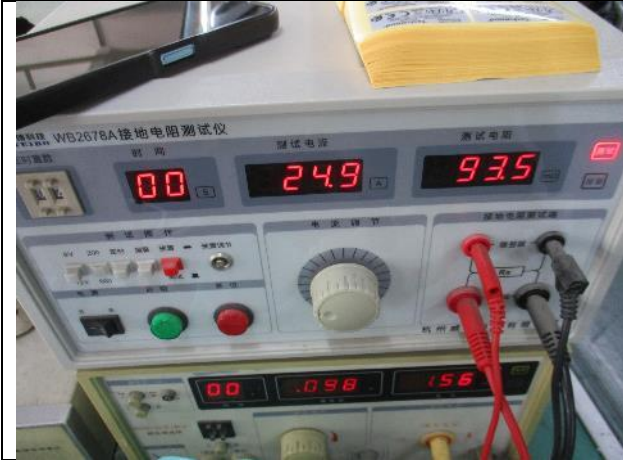
91. Earthed resistance test
