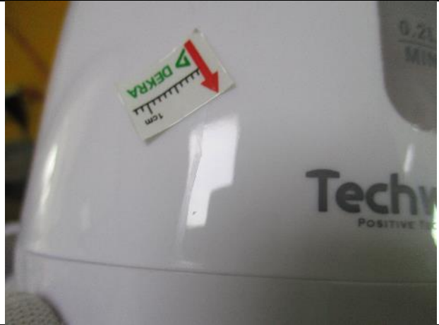
116. Scratch mark on surface
