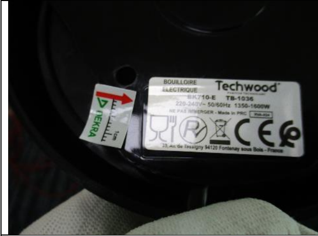
121. Poor stuck of the rating label
