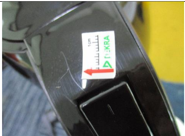
120. Scratch mark on surface
