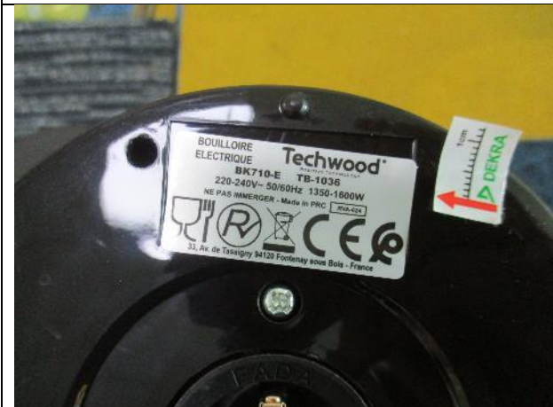
119. Poor stuck of the rating label
