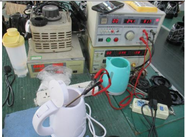
90. Earthed resistance test
