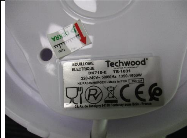
115. Poor stuck of the rating label
